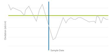
The graph above illustrates the improvements in the engine oil's Oxidation, where you can see the Oxidation results being well above the engine's condemning limit (green line) prior to the coolant conversion (left of the blue line), and how the Oxidation is comfortably below this condemning limit after the coolant conversion (right of the blue line).
